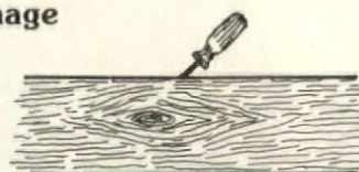
In advanced cases of termite infestation, a screwdriver can be driven deep into the wood.
