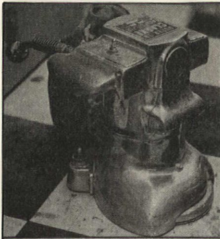
Left, the disc sander used for edges of the floor.
