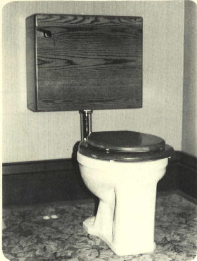
Tank size - 8"x19"Wx17½"H Bowl roughs in 12" from wall
