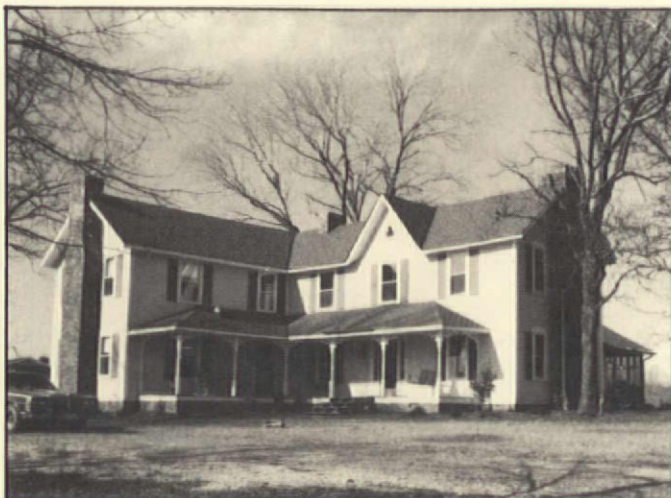
Harmony Hill today. Note the Gothic trefoil in the gable of the original structure and the scroll trim of the porch columns.
