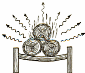
CONVENTIONAL GRATE—Heat radiates in all directions
