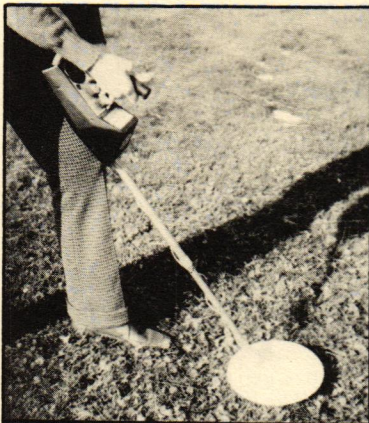
1. "Singing" of detector indicates metal beneath the surface.
