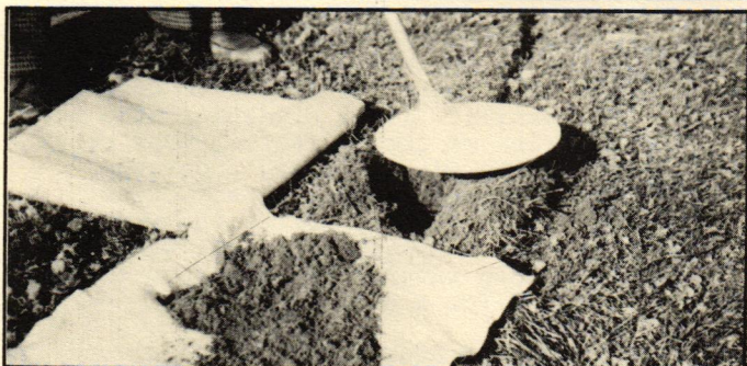
5. Continual scanning with detector over hole tells you when metal object has been removed with the dirt.
