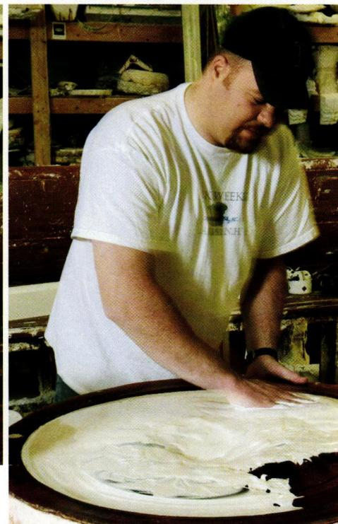
**STEP 2:** He then uses his hands to smooth it and work it into the deeper recesses. To effectively interact with water and become uniformly hard, gypsum powder must be fresh.
