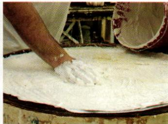
**STEP 4:** Sharpe applies another layer of plaster to completely encase the fiber.
