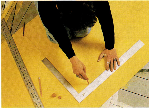
Marking the Border: Using a framing square, measure a 1" border in pencil. (Leave extra for the hem.) Make sure it is the same width on all sides. With chalk, draw a crisscross through the center of the field as a guideline when stenciling.
