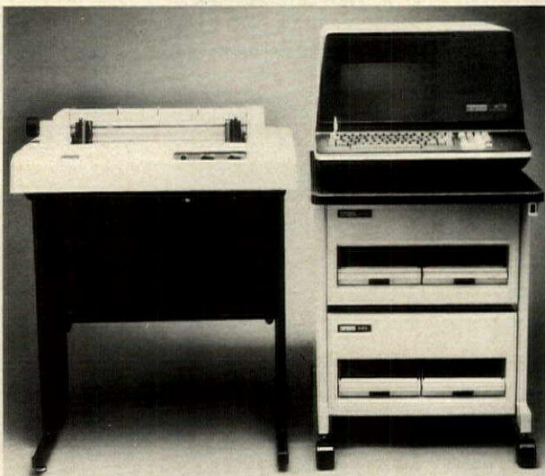
Construction management system (above) runs on the WS78 word/data processor shown above. The system—which includes job costing, accounts payable, accounts receivable and payroll modules—also includes such equipment as the video display terminal with keyboard, two dual-diskette drives, and a choice of printers. Digital. Circle 205 on reader service card
