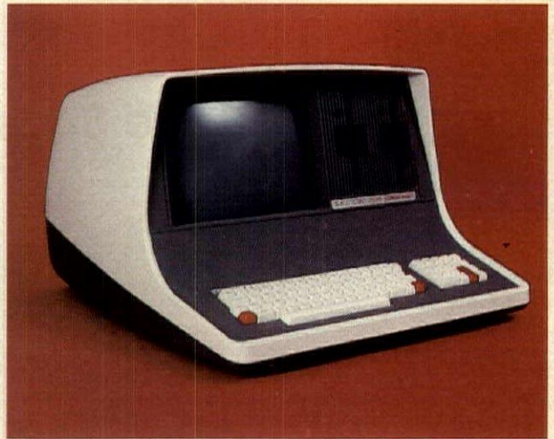
SuperBrain™ (above), a self-contained desktop computer, has two memory drives which can hold nearly 350K bytes of disk storage. Also featured is a CP/M® disk-operating system to insure compatibility with the wide variety of software available from manufacturers. Intertec Data Systems. Circle 209 on reader service card
