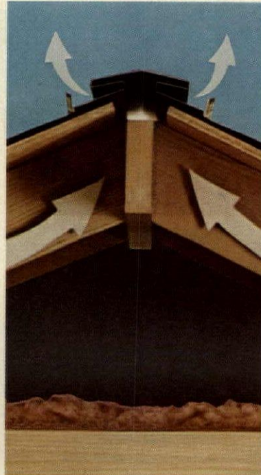
Vent-A-System*. It saves energy, but doesn't use energy. It cools your attic with natural convection and wind action.
