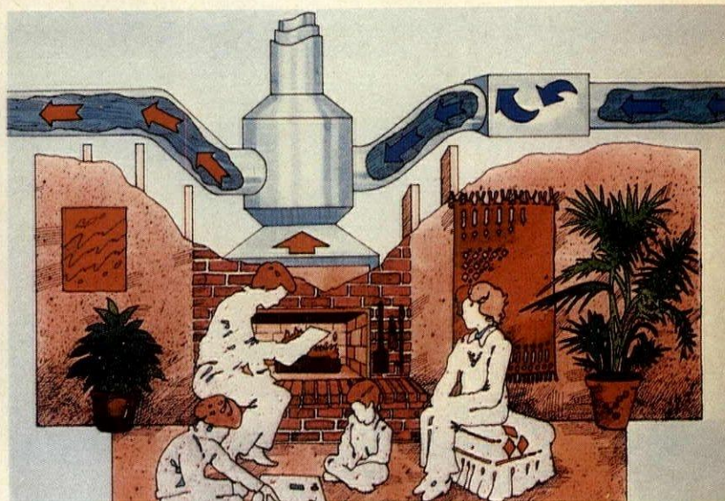
Forced-air fireplace/furnace (left) includes a heat exchanger, six-ft. flue section, insulation and glass doors with screen. Energy Savers. Circle 205 on reader service card
