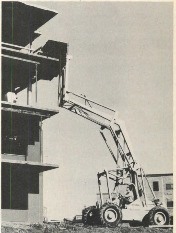
Forklift (above) has a maximum lift height of over 33' and a horizontal reach of up to 88''. Material-moving truck has a frame-leveling feature that can be hydraulically applied to keep loads level while crossing rough terrain. Hyster. Circle 275 on reader service card
