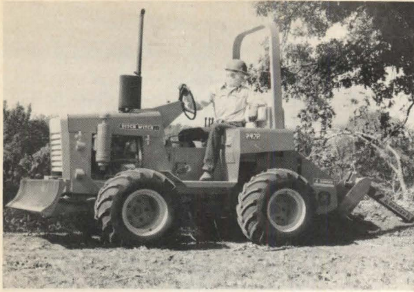
"Ditch Witch modularmatic" (above) incorporates an offset trenching and vibratory plow assembly in one module. The multi-purpose vehicle is available with a 30-hp diesel or gasoline engine. Rear steering is offered as an option. Charles Machine Works. Circle 270 on reader service card
