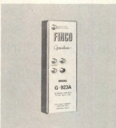
Solid-state distribution amplifier (above) has the capacity to handle four television sets. The 82-channel unit, designed for a 75-ohm system, has an FM trap-switch that eliminates interference from local FM radio signals without affecting television reception. Unit measures 8 1/2" x 3" x 1 1/2", and necessary hardware is included. Finney. Circle 255 on reader service card
