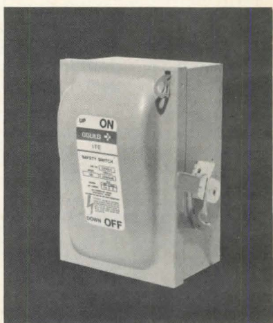
Wall-mount safety switch (above) can be used with 1/2- to 3-hp-rated motors. The switch will accommodate electrical systems that are rated 120v AC. It is offered in NEMA Type 1 and 3R enclosures. Gould. Circle 259 on reader service card
