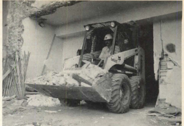
Skid-steer loader —measuring 75'' high and 55'' wide—is suitable for working in tight spaces like that above. Loader is part of the new "730" series and weighs 1,300 lbs. A single-speed transmission assures smooth operation between 0 to 6 mph. Clark. Circle 273 on reader service card
