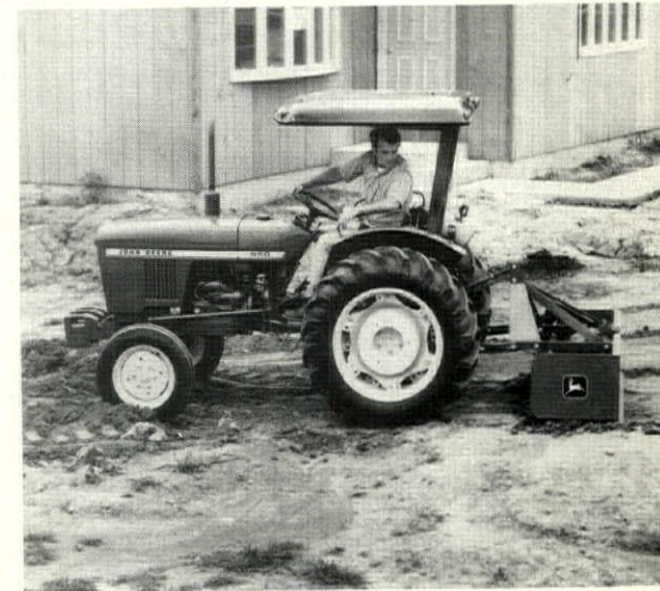
Compact tractor, "Model 950" (below) , is powered by a 3-cylinder, 27 hp engine. Vehicle has an 8-speed transmission with 2-lever control, and a differential lock that engages on the go. John Deere, Moline, IL. Circle 261 on reader service card
