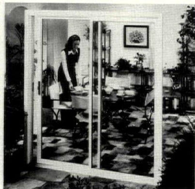
Wood patio door, ThermaSlide® (above), features tempered insulating glass. Inside movable panel prevents ice build-up and allows full closure of door against the weather. Factory-installed weatherstripping and "Dual Seal" interlock prevent air infiltration. Sills are heavy-duty aluminum and rollers are adjustable. Security lock is optional. Malta, Malta, OH. NAHB booth 2336. Circle 155 on reader service card
