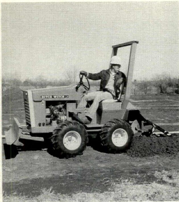
Riding trencher, "Model 2200" (above), is powered by an air-cooled heavy-duty 18 hp engine. Four-wheel-drive vehicle is capable of digging a trench from 4¼" to 12" wide to depths of 5'. Hydraulic backfill blade has 35° swing angle left or right. Ditch Witch, Charles, Perry, OK. Circle 172 on reader service card
