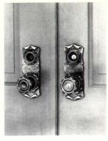
Multiple-security lock pair (above) is for double door entries. The functioning unit (right in photo) has a deadlocking latch and a 1" throw deadbolt. A turn of the inside knob releases both locks. Amerock, Rockford, IL. Circle 229 on reader service card
