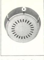
Smoke and fire detector, Earli-Gard® (above), is a solid state ionization-type unit. Up to six direct wired units can be interconnected to sound simultaneously. Unit has universal mounting bracket. Square D, Lexington, KY. Circle 230 on reader service card
