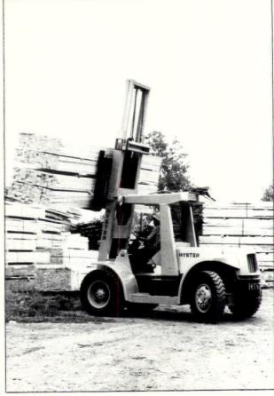
Lift truck (above) is part of the "Challenger" series. Units in the pneumatic-tire line have capacities ranging from 15,000 to 27,500 lbs. at 24" load center. Vehicle has hydrostatic steer axle and shock-absorbing seat suspension. Hyster, Portland. OR. Circle 234 on reader service card
