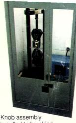
is pulled to breaking point on hydraulic tensile-test unit to insure that product meets strength specifications.
