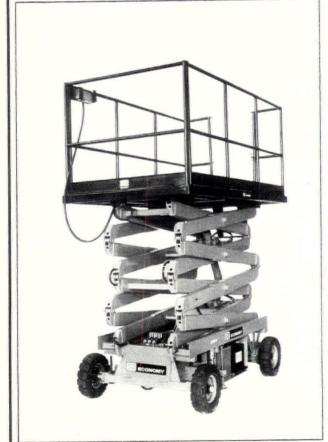
Driveable work platform (above) features dual-wheel hydrostatic drive and forward and reverse speeds. Unit has control panel on platform for driving, turning and raising and provides working heights to 26'. Economy, Bensenville, IL. Circle 241 on reader service card
