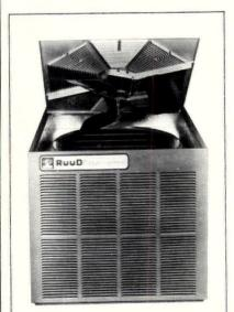
Remote condensing unit (above) has 10.0 and 10.3 EER in the 2- and 3-ton capacity. Standard features: start components, compressor time delay and pressure controls. Ruud, Fort Smith, AR. Circle 269 on reader service card
