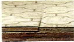
Regular flooring can crack or ridge.
