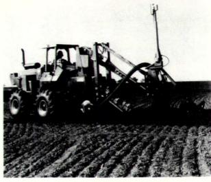
tiling attachment (above) installs plastic drain tubing up to 8" in diameter at depths to 6'. Device molds bottom trench for proper tile bedding. Ditch Witch, Perry, OK. Circle 259 on reader service card
