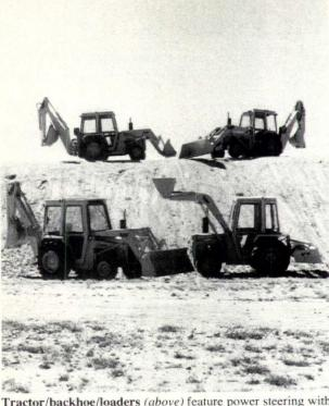
Tractor/backhoe/loaders (above) feature power steering with manual pump back-up. The units, with short turning radiuses, have breakout forces from 4500 lbs. to 8700 lbs. Massey-Ferguson, Des Moines, IA. Circle 248 on reader service card
