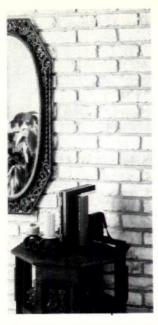
brick Simulated panels (above) are easy to install with nails or adhesive. Lightweight 6- or 12-brick panels come in shades of brown, beige and rust. Marlite, Dover, OH. Circle 223 on reader service
