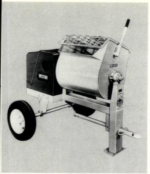
Mortar/plaster mixer (above) has a 51/2 cu. ft. capacity. Unit features "two-in-one" blades-a regular steel blade for abrasive mixes is mounted over a full removable rubber blade that acts as a squeegee. Stow, Binghamton, NY. Circle 249 on reader service card
