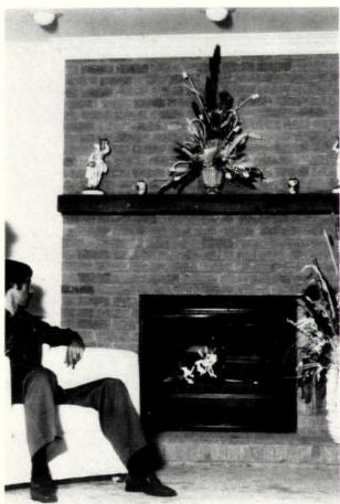
Fireplace, "Energy Mizer" (above), is a wood-burning, heatproducing unit designed to conserve fuel. Cool room air is drawn into a heating chamber completely sealed off from the firebox, warmed and recirculated. Preway, Wisconsin Rapids, WI. Circle 228 on reader service card
