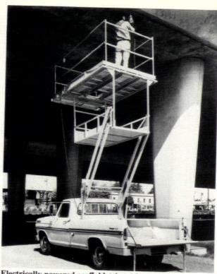
Electrically powered scaffold (above) has movable push-button controls. Unit with a 24' reach and a 1000-lb. capacity has a skidproof aluminum platform. Up-Mobile, Sacramento, CA. Circle 254 on reader service card.
