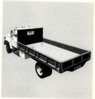
Heavy-duty steel contractor truck body (above) features a 4-way double-hinged tailgate and extra cross sills for heavier load handling. Bodies come in 12', 14' and 16' sizes with smooth or deck-plate steel or 2" wood floors. Reading, Reading, PA. Circle 260 on reader service card
