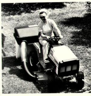
"Broadmoor II" garden tractor (above) is available with a rear-mounted grass catcher as shown. Mower has a choice of five cutting heights ranging from 1½" to 3½". Simplicity, Port Washington, Wis. Circle 362 on reader service card
