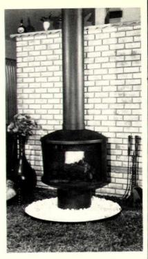
"Wigwam" Freestanding fireplace, (above), is a contemporary-style unit offered in 30" and 36" diameters. Unit with steel firewalls and sidewalls requires a 22" clearance from combustible walls in a corner installation and 16" clearance for flat wall application. Ember Box, Oklahoma City, Okla. Circle 304 on reader service card
