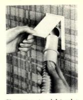
Vacuum system inlet valve (above) is made of crack-, and rust-resistant Lexan®. Lifting the valve cover activates system. To allow enough room for connecting hose, cover opens 180°. H-P, Louisville, Ohio. Circle 315 on reader service card
