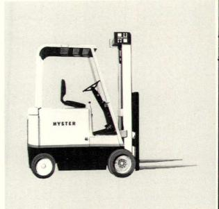
Electric-powered sitdown lift truck, "E40B" (above), has a 400 lb capacity at 24" load center. A single Monotrol® pedal controls acceleration, forward and reverse direction and braking. Frame is welded, all-steel, one-piece construction. Hyster, Portland, Ore. Circle 351 on reader service card
