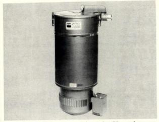
Heavy-duty built-in vacuum (above) simplifies maintenance of apartment and commercial buildings. "No. CS-250" with a 9.5-amp power consumption has a positive filtering method including paper bag, cloth bag and a flocked wire filter. VSI Filtex, Temple City, Calif. Circle 318 on reader service card
