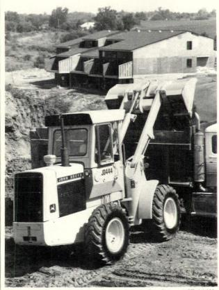
Compact 4-wheel drive articulated loader, (above) has all the features of larger models. Vehicle is equipped with a power-shift transmission, wet-disk power breaks, power steering, a single lever loader control and a ROPS canopy. John Deere, Moline III. Circle 347 on reader service card
