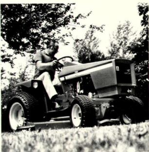
Lawn and garden tractor, "Model 720" (above), features a hydrostatic drive system. Front and rear PTO's accommodate the full range of attachments available. Accessories include mowers, a tiller, a plow, a snowthrower and a loader. Allis-Chalmers, Milwaukee. Circle 359 on reader service card
