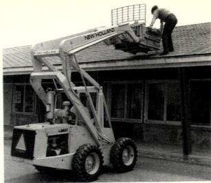
Skid-steer loader (above) features a patented boom. The higher the boom rises, the farther forward it reaches, permitting dumping into tandem-axle-trucks or over walls. Sperry New Holland, New Holland, Pa. Circle 348 on reader service card
