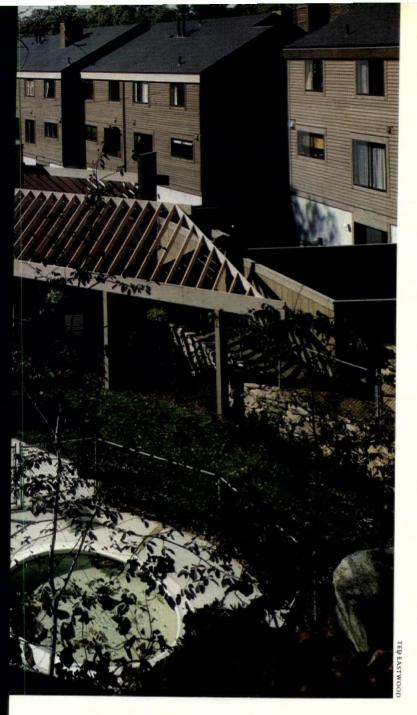
**80-ft. buffer** required by zoning *(green area on site plan below)* forced the units to the center of the 13-acre site. Parking was brought to the front of the units so that the rear could be used for private yards, most of which open onto the heavily wooded buffer. Some 2,000 additional trees are being planted among the buildings to insure that the linear plan does not result in a tunnel effect.
