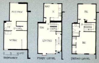
1,153-sq.-ft. Fitch model was designed for young people stretching to make the move from apartments. It has only one bath but was designed so that a lavatory could easily be added (in the space where the dining table is in photo at left). This proved to be unnecessary; the market accepted it as is. Fitch prices opened at \$39,900; the final price was \$44,900.
