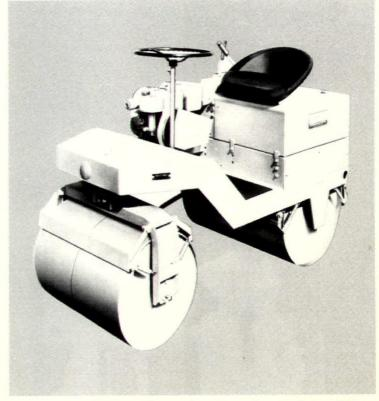
Roller, "Econoroll" (above), features low-center-of-gravity design which enables it to perform on steep grades and slopes. The offset compression roll allows for close-up work without special added attachments. Stow, Binghamton, N.Y. CIRCLE 259 ON READER SERVICE CARD
