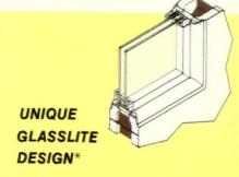
Factory installed insulated tempered glasslite with attractive recessed aluminum trim.
