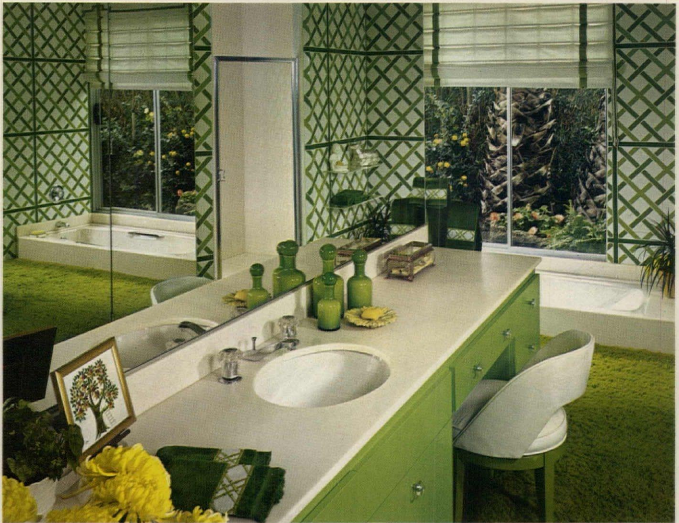
Master bathroom has long vanity tops of solid, 3/4" Cameo White CORIAN. Shower surrounds, whirlpool tub trim and side and back splashes are in 1/2" Cameo White CORIAN.
