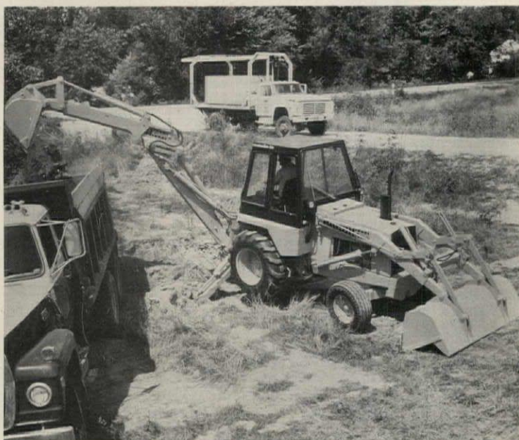
Backhoe loader "580 Construction King" (above), has a shock-absorbing unitized main frame. A componentized power train makes for easy servicing. Unit is equipped with a 14' standard backhoe. J.I. Case, Racine, Wis. CIRCLE 262 ON READER SERVICE CARD
