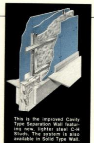
struction meant quicker sales and less construction loan interest. Based on EME's own cost analysis, the U.S.G. system, which had a 2-hour fire rating, 53 STC sound control rating and 41/2" thickness, cost \$150 less per unit than a comparable block assembly of 11" thickness!
