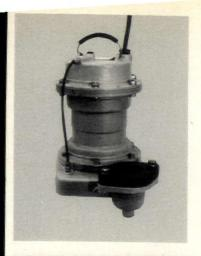
Cast-iron sewage pump, "Model T-22" (left), features dual mechanical shaft seals for maximum reliability. Heavy-duty submersible pump has capacity of 6600 gallons per hour at a 10-foot head. Kenco Pump, Lorain, Ohio. CIRCLE 251 ON READER SERVICE
