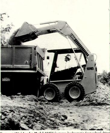
Compact "Uni-Loader Model 1845" features hydrostatic four-wheel drive Engineered for high-production loading and material handling, unit has the ability to spin-turn in its own length. J. I. Case, Racine, Wisc. CIRCLE 258 ON READER SERVICE CARD
