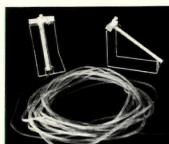
Lightweight surveying instrument "Leveller," can be easily used by one person. Elevation differences are re corded on two calibrated stands linked by a flexible plastic hose filled with water or other fluid Forrgley, Los Angeles. CIRCLE 262 ON READER SERVICE CARD
