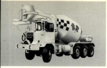
ront-discharge truck mixer, "Vanuard," with a 9-11 cu. yd. capacity ombines the operating advantages if forward placement and the perormance efficiency of a rearischarge drum configuration. Unit eatures Gyro-Drive®. T. L. Smith, Marion, Ohio. CIRCLE 263 ON EADER SERVICE CARD
