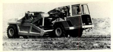
High-volume scraper, "JD762," is a versatile machine with two-axle design. Powered by a 175 hp diesel engine, vehicle has a power shift transmission and a top travel speed of 28 mph. Roll-over protective structure is a standard feature. John Deere, Moline, Ill. CIRCLE 252 ON READER SERVICE CARD
