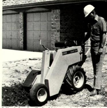
Rubber-tired trencher, "Fleetline 7-2," is equipped with a 7hp Briggs & Stratton air-cooled engine. It trenches at speeds from 1.8 fpm to 4.8 fpm with a 3.6 mph transport speed. The two-wheel drive unit digs from 4"-6" wide and 24" deep. Davis. Wichita, Kans. CIRCLE 262 ON READER SERVICE CARD
