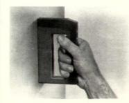
Hand-held metal detector, "Sensor matic MkI," has double the sensi tivity of its predecessor. The unit lo cates hidden nails, wires, pipes, con duits, reinforcing bars, etc. An metal in the tool's magnetic field produces an unbalance in a bridge circuit, indicated by a light. Na tional Instrument, Baltimore CIRCLE 260 ON READER SERVICE CARD
