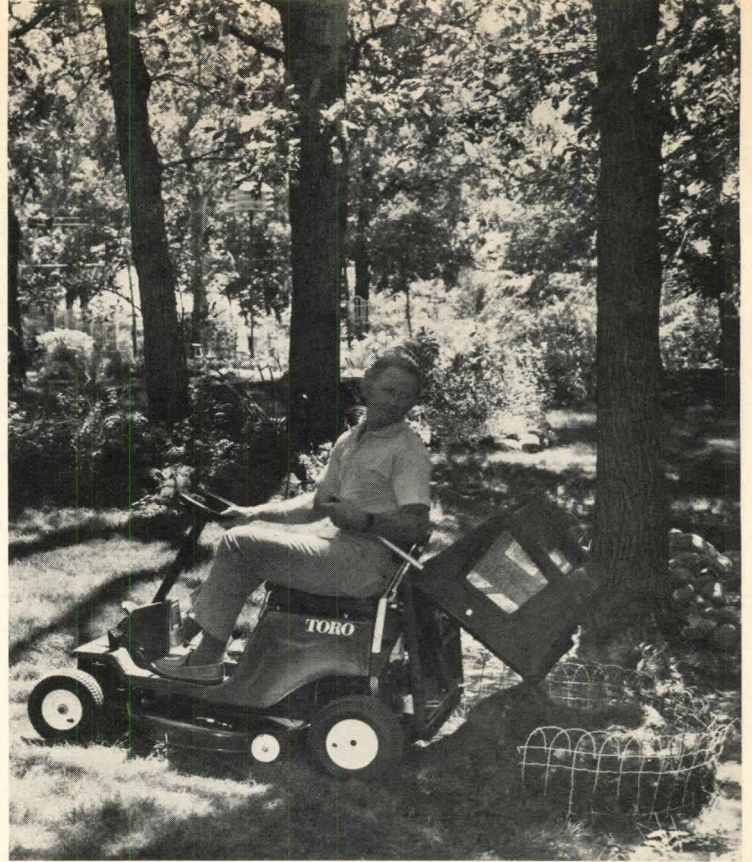
"Whirlwind Premium Rider" mower features an easy-to-empty grass catcher as an option. The rear-engine unit is available in a 5 hp model with a recoil start or in a 7 hp version with an electric starter. Mower cuts a 25" swath. Toro, Minneapolis, Minn. CIRCLE 265 ON READER SERVICE CARD
