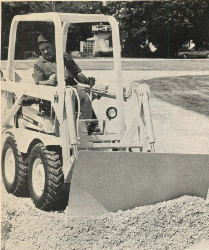
Highly maneuverable skid-steer loader-tractor turns a full 360°. Unit has hydrostatic transmission, 4-wheel drive and ground-hugging oscillating axles for better traction. A wide range of quick-attach tools is offered. International Harvester, Chicago. CIRCLE 262 ON READER SERVICE CARD
