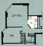
The diagonal wall that separates this compact, L-shape kitchen from the living area provides privacy without creating a closedin feeling. Using this type of partitioning instead of the typical right-angle wall allows a dining table to be placed inside or outside the kitchen. Openings at wall ends are wide enough to permit a free flow of traffic.
