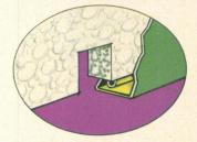
Moisture control notches spaced every 311/2" in foam insulation board . . . help dissipate trapped moisture.
