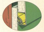
Thermal break . . . top ridge of aluminum rests on foam insulation, breaks metal to metal contact, prevents air infiltration.
