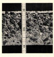
Epoxy sealer, "688," penetrates as much as 2" (as above) into untreated concrete surfaces before hardening. Brush-, roller- or spray-applied sealer provides resistance to chemicals that cause decomposition. Ceilcote, Berea, Ohio.
