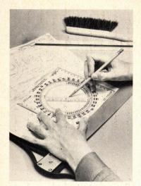
Protractor square, ROTANGLETM, (left) provides readings as precise as 0.1°. Any angle to 360° may be dialed and a line drawn through the vertex without changing position. Acrylic device is calibrated in inches and centimeters. Labindustries, Berkeley, Calif.
