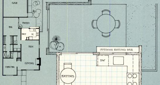
In this plan a pass-through window, an outdoor eating bar and sliding glass doors contribute to the feeling that the indoors and outdoors are one. Even the eatin section of this kitchen is oriented to the outdoors. This compact plan shows that the in-
