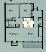
One wall of this windowless corridor kitchen has been opened to the dining area. This permits serving directly from the preparation area and also keeps the kitchen private without isolating it as a solid wall would. With this kind of arrangement, cabinets can be hung so that they either help
