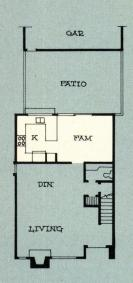
In a plan like this, where family-room space is limited, a bar-height divider serves as the informal eating area, eliminating the need for a table in the family room. This kind of arrangement is especially important when the formal dining room is an extension of the living room, as it is here. Note also the pass-through window on the sink-dishwasher wall which links the kitchen directly to the outdoor living area.
