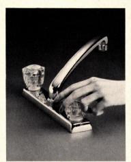
Water-controlling device, "Flow-Matic," offers temperature and volume selection with a single handle. Fitting has ceramic cartridge that eliminates need for lubrication or washers and requires no "O" rings. Price Pfister, Pacoima, Calif.
