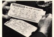
Metric/inch converter in handy slide-chart form is used to translate U.S. units of measurement into metric units. Interchange between 35 metric and U.S. units is provided, including lengths, weights, volumes and areas. Plastic-coated calculator is small enough to fit in a shirt pocket. Jaydee, Wilmette, Ill.
