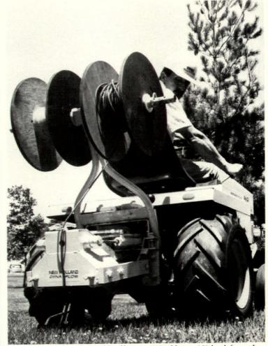
Line-laying machine is capable of burying 3%" cable to a 10" depth faster than trenching units. The "Model T-220 Dyna-Plow" uses a vibrating blade that knifes through the ground rather than digs. Cable is fed from reels into the narrow slit created by the blade, causing less lawn damage than a trencher. Sperry New Holland, New Holland, Pa. CIRCLE 256 ON READER SERVICE CARD
