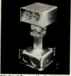
Poke-through floor assembly, "Fire-I Model 300-21," complies with NEC requirements for prevention of fire spread. Palusol™, a fire-rated chemical used in the center coupling, forms a thermal insulating foam barrier at excessive temperatures. Factory-assembled unit fits 2½" to 8" concrete floors. Raceway Components Inc., Linden, N.J. CIRCLE 245 ON READER SERVICE CARD
