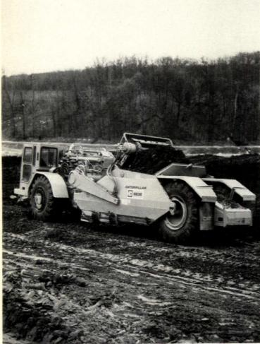
Improved elevating scraper has a variable-capacity torque converter. Operator can control the amount of horsepower directed to the wheels so that the maximum is available to the hydraulic system for elevator operation. Unit, with increased steering angle, has cushion-hitch feature that reduces stress. Caterpillar, Peoria, Ill. CIRCLE 250 ON READER SERVICE CARD
