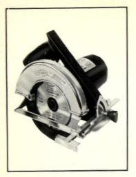
Roller-bearing 71/4" circular saw is powered by a 2 hp, 12 amp, 5100 rpm motor. Lightweight unit is built with double insulation and a unitized motor. Saw features a chrome-plated guard and base assembly and a chrome-nickle combination blade and rip guard. Wen, Chicago.
