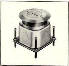
"F4000" self-leveling floor boxes save installation time and cut the need for grouting. The tiltable top flush-mounts to floor or carpet at levels up to 10° from the horizontal. Wide shoulders conceal box and carpet edges. Three knockout patterns are available. Bell, Chicago, Ill. CIRCLE 246 ON READER SERVICE CARD
