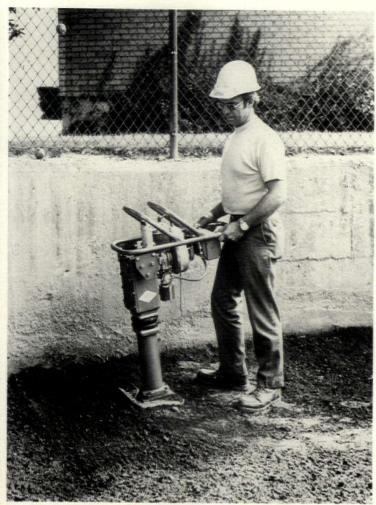
Rammer tamper hits with an impact of 1,750 lbs. per blow, 700 times a minute. Powered by a 4.5 hp, 2-cycle engine, unit features a shock-mounted handle and a completely sealed, oil-bath lubrication system. Designed to be used by one man, the tool comes with a standard 11"x12" steel shoe. Stow, Binghamton, N.Y. CIRCLE 259 ON READER SERVICE CARD.
