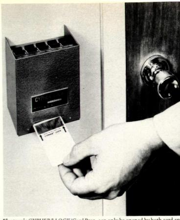
Electronic CYPHER® LOCK/Card Prep, can only be opened by both card and pushbutton code. Housing is mounted outside the protected area. Once card is inserted and correct four-digit code tapped out, door unlocks for a set, adjustable period of time. System can activate an alarm. Continental Instrument, Hicksville, N.Y. CIRCLE 219 ON READER SERVICE CARD
