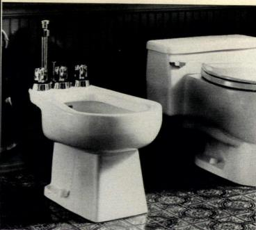
Vitreous china bidet, "Carmen," can be ordered with or without a standard fitting. Chrome-plated, three-valve set has a transfer valve to direct tempered water to a fountain spray-head in the center of the bowl. Unit comes n eight colors. Briggs, Tampa, Fla. CIRCLE 209 ON READER SERVICE CARD
