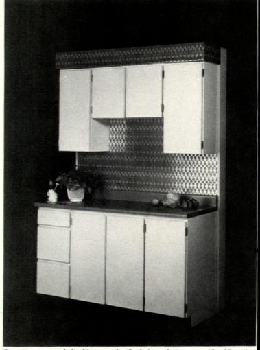
**Contemporary styled cabinets** with a flush-front design are made of Formica in a solid-white, suede finish. Features include full-height base-cabinet doors and drawer banks with side-mount, ball-bearing track. Upper cabinets have one adjustable and one fixed shelf. Self-closing hinges are standard. Villa, Mfg., Rochester, N.Y. CIRCLE 211 ON READER SERVICE CARD
