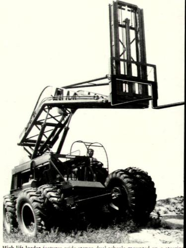
High-lift loader features wide-stance dual wheels mounted on a steering axle. Loader, with a 130" span to the outside of the dual wheels, provides maximum stability and mobility. Designed for use with a 41½" lift, loader also can be used with other models. Outer wheels are removable for road transport. Lull, St. Paul, Minn., CIRCLE 267 ON READER SERVICE CARD
