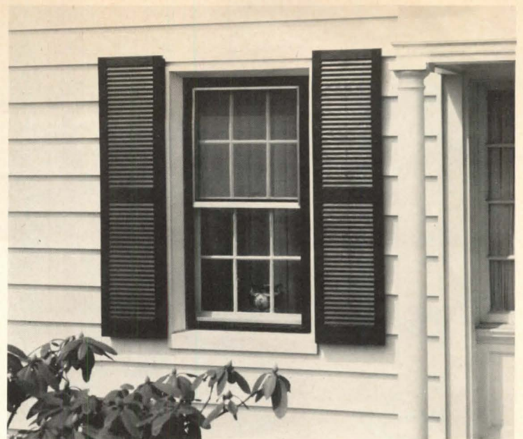
Decorative shutters with a deep wood-grain texture are molded of high-density polystyrene. Offered in white, black, brown, avocado, forest green and barn red, the open louver shutters can be painted if desired. Easy-to-install 15"-wide units come in 11 lengths ranging from 36" to 80". Certain-teed, Valley Forge, Pa.
