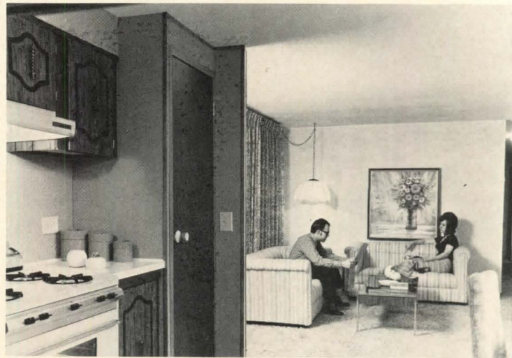
Outward-bound Steelbond unit leaves one of DMH's two newly converted plants in Alma-St. Louis, Mich. (above). Inside the new units (right), light-colored, vinyl-faced gypsum panels have replaced the woodgrain wall panels found in conventional mobile homes. The new look, say company officials, provides a more spacious appearance and gives owners greater latitude in decorating.
