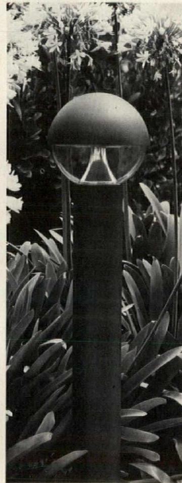
Outdoor bollard , has a 10" clear acrylic diffuser sphere with a spun aluminum reflector. "Transhemisphere," a post-mounted fixture, provides low-brightness lighting. Finished in textured black, the lamp with concealed mounting rests on a 5" diameter post of heavy-duty aluminum. Unit comes in 100W mercury vapor or incandescent models. Prescolite, San Leandro, Calif. CIRCLE 236 ON READER SERVICE CARD
