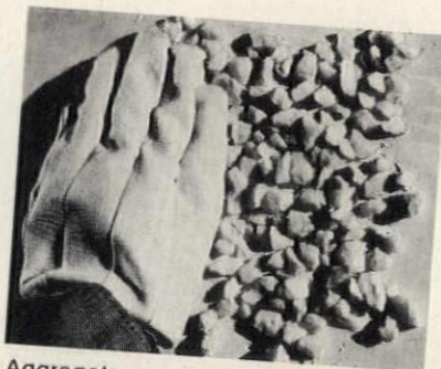
Aggregate can be hand-seeded in the field or mechanically applied in the shop.
