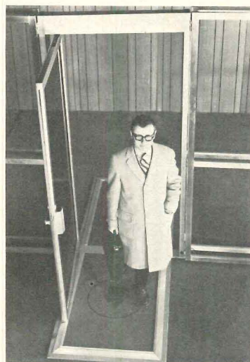
Automatic door opener converts most doors. Visible "Monopack" installs over transom; concealed unit replaces transom. Both run on \frac{1}{4} -hp. electric motor. Floor carpet (or pull cord, pushbutton, push or kick plate, or floor button) opens door 90°. Hydraulic spring closes. Stanley, Farmington, Conn.
