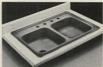
Double sink is a self-rimming unit called Flex-Vit. Made of steel, it has a hard enamel coat applied by a new process. Sinks also come in stainless, brushed or smooth, with single control faucets and stainless basket strainers. Federal Stainless Sink, Bloomington, Ill.
