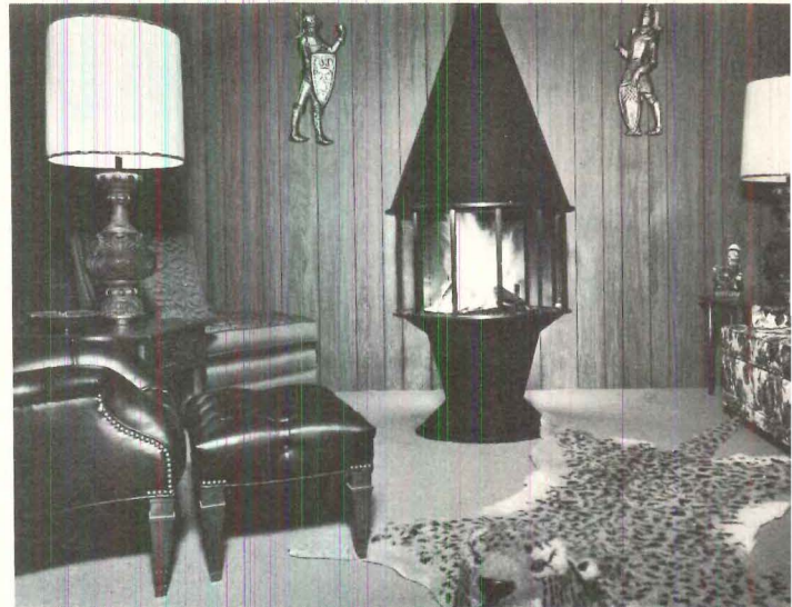
Circular unit , through baffles in hood, spins flame around and up the flue with a strong draft that lifts 90% of ashes up and out. Hearth rarely needs cleaning. Intensity of flame efficiently burns
