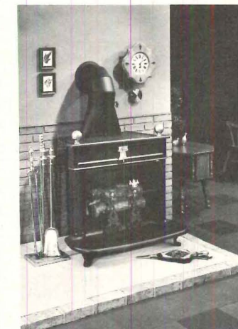
Franklin stove burns wood, charcoal, or gas or electric logs. It is hand-poured of cast iron, comes equipped with basket screen, inducer with damper, brass knee elbow. Width is 33½", height (with legs) 37½", depth 13½". Black or U.S. Stove, South Pittsburg, Tenn. CIRCLE 307 ON READER SERVICE CARD
