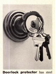
ball in the tumbler that allows one key to operate during construction. A second key allows ball to be withdrawn by a magnet, so only the third—homeowner's—key will operate lock. Weslock, Los Angeles.
