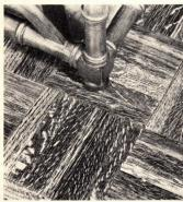
**Treated wood** is ordinary red oak, given extra toughness by impregnating it with resins under pressure, then curing the resins within the wood by gamma ray bombardment. The wood is then backed with plywood. American Novawood, Lynchburg, Va. Circle 302 on Reader Service card
