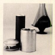
Prefab chimney can be used with freestanding fireplaces or as an outside chimney. Construction is double-wall stainless steel, with 1"-thick insulation. Pipe sections will lock together with a simple twisting motion. Wm. Wallace, Belmont, Calif.
