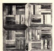
**Teak flooring** is a luxury wood incorporated into three distinctive patterns in 5/16"-thick tiles. Two are 12" x 12", and the third is 9" x 9". Kiln-dried, prefinished, and felt-backed, all have fine sanded, eased edges. Plywood International, Brooklyn, N.Y.
