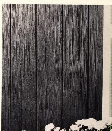
Hardboard siding has a gnarled, deeply textured, barklike surface. Panels, 4'x8' and 4'x9', have ½"-wide square-cut vertical grooves on 8" centers. Lap siding, 12"x16', has horizontal texture. Primed or unprimed. Masonite, Chicago. Circle 352 on Reader Service card
