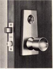
**Double lock** for extra security combines a regular lock with a special 1"-throw deadbolt that has a roller bearing so it can not be sawed through. A one-handed single twisting action will open door instantly from inside. Schlage, San Francisco.
