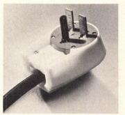
Angle plug for tight areas, this two-pole, three-wire plug can be mounted in any of four directions from a fixed outlet. Pressure-type terminals make wiring quick and easy. Made in white nylon with arc-resistant plastic face. Bryant, Bridgeport, Conn.
