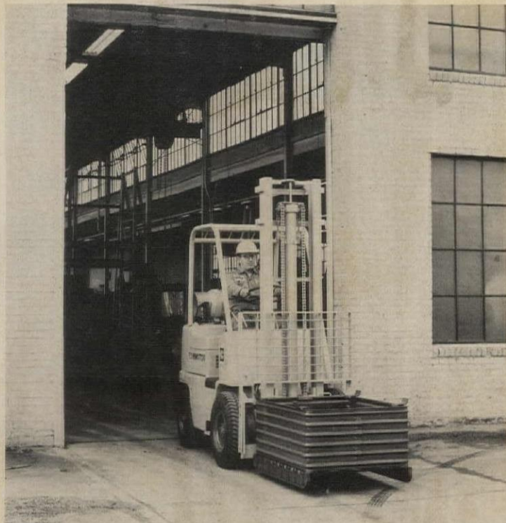
Fork-lift truck is one of a new ten-model line with capacities of 3,000 to 6,000 lbs., solid or pneumatic tires. New features: adjustable contoured seats, self-lubricating wheel bearings. Towmotor, Cleveland, Ohio. Circle 229 on Reader Service card
