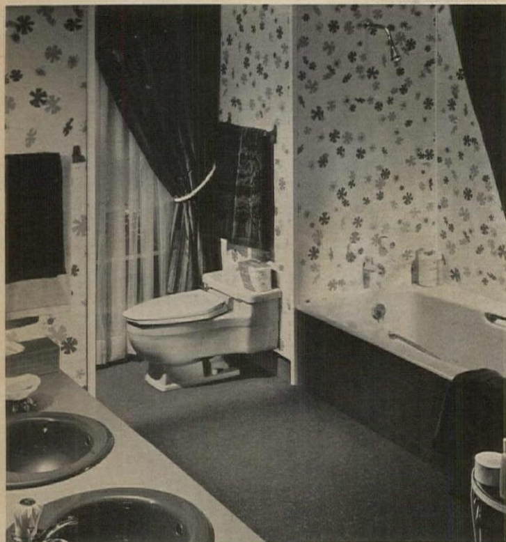
Moisture-proof panels have a decorative laminate surface on an expanded polystyrene core, can be applied to any existing wall, including tile. Panels come up to 5'x10' in 18 patterns. Formica, Cincinnati, Ohio. Circle 203 on Reader Service card
