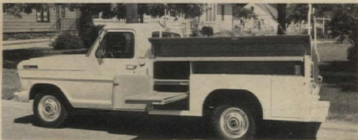
Flip-top door over the top compartment on the service-maintenance body offers storage space for material 6' to 9' long. Two more locking compartments are built into each side of pickup truck. Pierce Auto Body Works, Appleton, Wis. Circle 230 on Reader Service card
