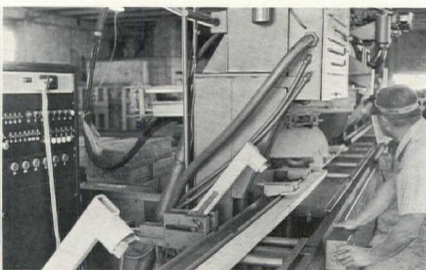
headquarters. Tapes actuate saw (right), which cuts truss members in dealer's or builder's plant.
