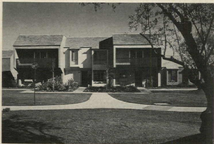
INDIVIDUALIZED DETAILING shows in this four-unit block of houses where several combinations of window shapes and placements are used.
