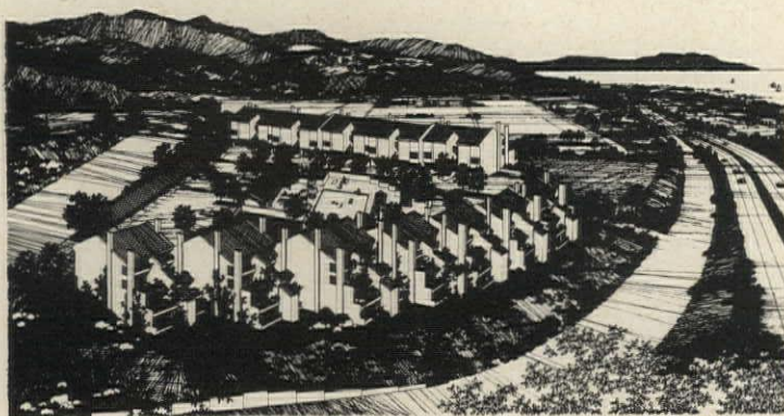
HILLTOP PLAN has recreation and parking on flat central pad. Townhouses are set around the rim of the hillside facing out toward view.
