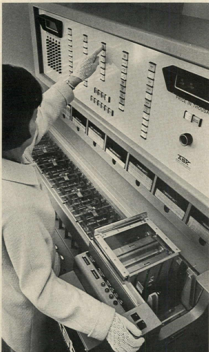
REAL ESTATE COMPUTER stores house listings in an NCR card-sorter, and salespeople retrieve them by selecting house features on pushbuttons.
