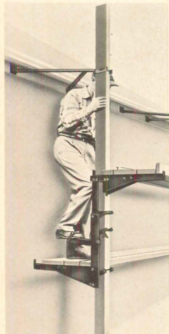
Scaffold adjuster is foot-operated, load-tested to 2,000 lbs. It attaches to an upright made of two 2x4s, and is secured by two gripping devices per upright. An optional workbench can serve as guardrail. Hoitsma, Patterson, N.J. Circle 264 on Reader Service card
