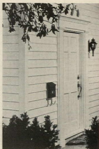
Narrow lap siding —in 18th Century Virginia style—has 5" exposure and measures 6"x16"x 7/16". Siding has slightly notched and contoured profile for a deep shadow line. Guidelines position adjoining laps and face nailing. Masonite, Chicago. Circle 206 on Reader Service card
