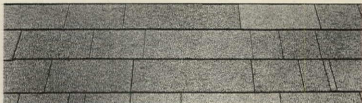
Double-surfaced asphalt shingles in nine colors are said to simulate thick-butt wood shingles. Embossing produces random vertical shadow lines. Dimensions: 5" exposure, 2" headlap, 36" length. Bird & Son, East Walpole, Mass. Circle 208 on Reader Service card
