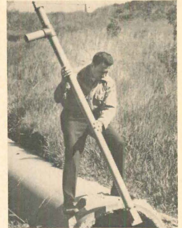
Long hand pump —for removing liquids from post holes, catch basins, and underground utility vaults—has a pumping length of 6' and removes a gallon of liquid with each stroke. Constructed of polyvinyl chloride. Beckson, Bridgeport, Conn. Circle 214 on Reader Service card
