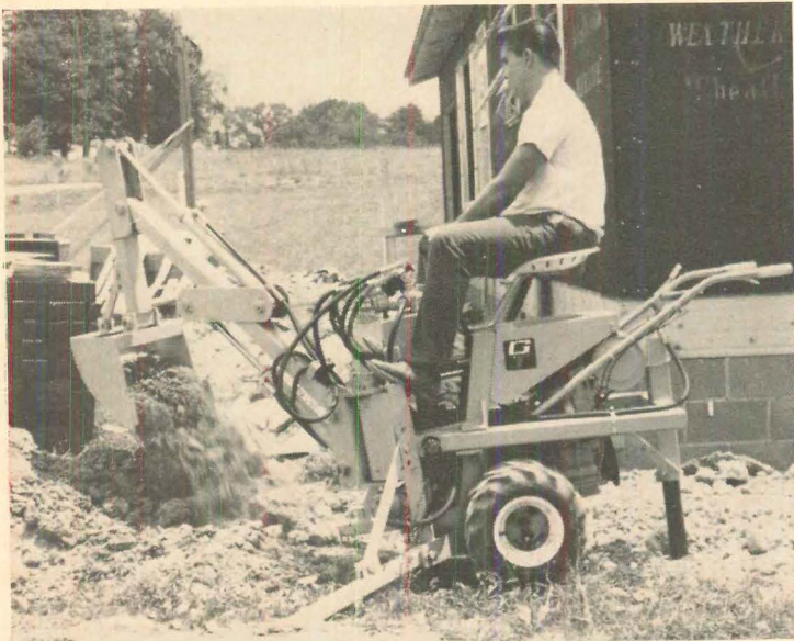
Compact backhoe for narrow places digs a 5'6"-deep trench 16" wide, and weighs slightly more than 1,000 lbs. so it can be transported on a pickup truck. Controls are operated by hydraulic pump. Gravely, Dunbar, W. Va. Circle 212 on Reader Service card
