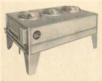
Air-cooled condenser for low-silhouette roof-mounting comes in two sizes with direct-drive fans. Unit consists of three fans with independent motors, and two-section condenser coil. For 7½- to 30-ton air-conditioning. McQuay, Minneapolis.
