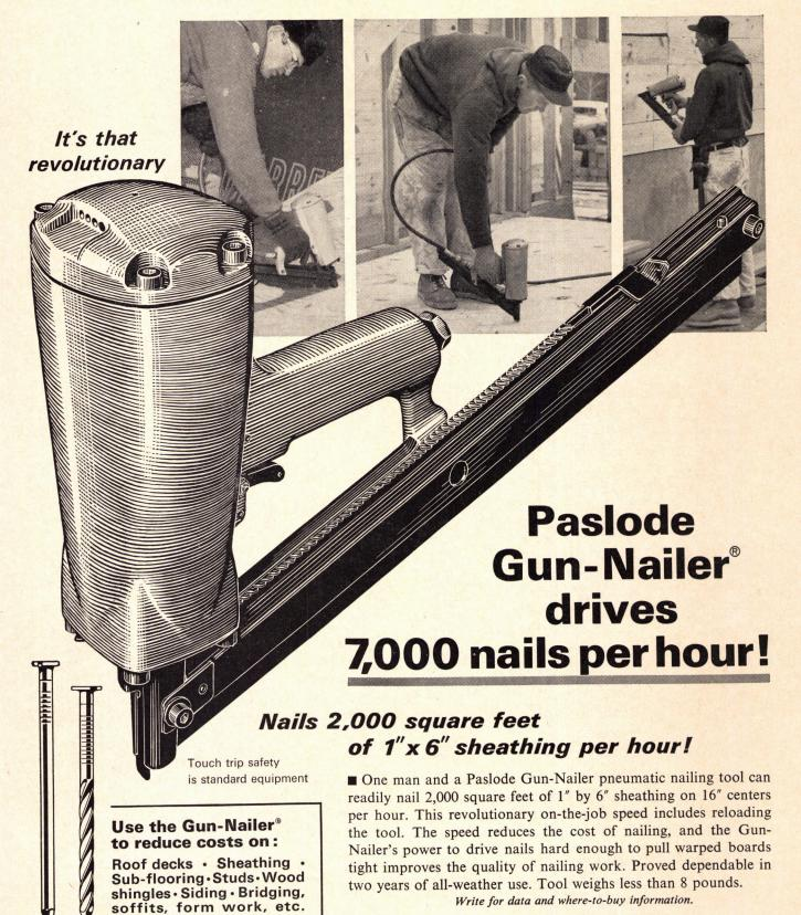
The Gun-Nailer drives regular 8d common or cooler and 6d common or cooler nails, with heads slightly modified to nest in clips. They are acceptable in FHA insured construction as equivalent to regular nails. They are *not* T-nails. It also drives galvanized nails 8d or 6d common; screw nails  $2\frac{1}{4}$ " or 2" long; short  $(2\frac{1}{8})$ " 10d nails for diaphragm roof and shear wall construction.
