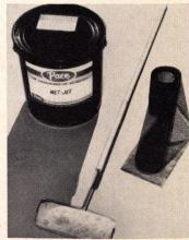
Roof coating can be applied in freezing temperatures or in rain or snow. Wet-Jet, a gilsonite liquid, is rolled on at the rate of 1½ gals. per 100 sq. ft. for composition and metal; 3 gals. per 100 sq. ft. for gravel. Pace, Kansas City, Mo.
