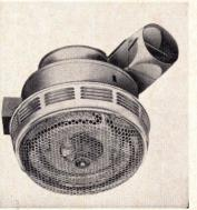
Heater and ventilator for bathrooms has mirror-finished aluminum grille and reflector. Infra-red wide-angle heated air is distributed by a permanently lubricated motor. Heating element is 1250 watts. Leigh Products, Coopersville, Mich.
