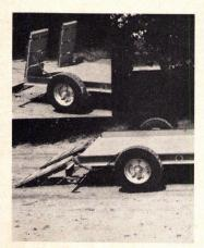
**Trailer** allows low angle loading with fold-up ramps and a low-profile ground clearance of 12". Trailer is 8' wide, 15'3" long and has a 10'2" oak deck. The model weighs 2½ tons. Brakes are electric. General Engines Co., Thorofare, N.J.
