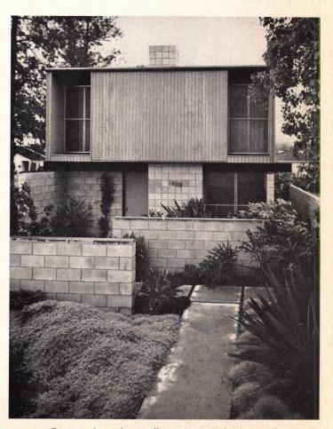
Staggered garden walls and an S-shaped walkway decrease the apparent depth of a 24' front setback (view B in plan). The walls also add privacy to the front entrance and living room courtyard. A 3' upper-level overhang shelters both the entrance and the court.
