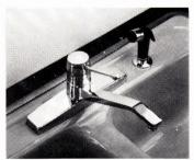
**Sink fitting** has a single lever that moves up to control water volume and from left to right to regulate temperature. The spout is cast brass and the working mechanism is a replaceable cartridge. A hose spray is available. Kohler, Kohler, Wis.
