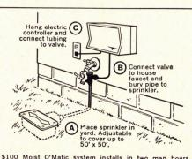
\$100 Moist O'Matic system installs in two man hours. Sprinkles up to 50' x 50' area. Additional sprinklers can be operated from electric control center for greater coverage. can install a system covering 50' by 50' (see illustration) in two man hours, the system shown above in less than eight man hours. No special plumbing or electrical work required.
