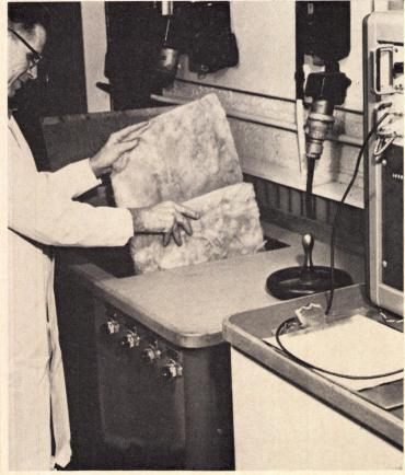
MOISTURE-ABSORPTION of insulation is checked at Owens-Corning lab.
