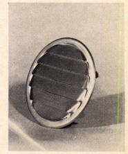
Small louver is designed to combat paint blistering and peeling, rotting and warping of wood and corrosion of metal. Units are available in six sizes from 1" to 4" in aluminum, copper and chrome. Midget Louver Co., Norwalk, Conn.
