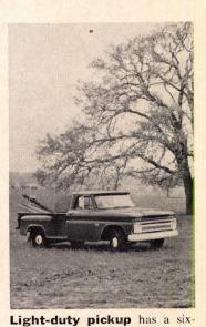
cylinder, 155 hp engine. Standard equipment includes seat belts, windshield washers, backup lights and corrosion-resistant brake lines. Three larger engines are also available for the same model. Chevrolet, Detroit.
