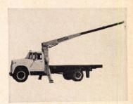
Hydraulic crane rotates 360° in either direction. Unit elevates to 85° to 90° and loads over front, rear or sides with single or double line. Flex-Lift requires 14" of frame space. It has two self-centering levers. P-M Machine Co., Bryan, Tex.
