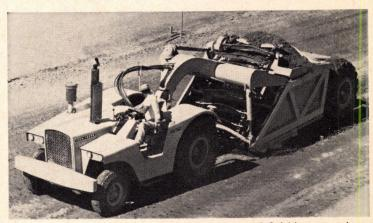
**Scraper,** designed for primary earthmoving and finishing operations, allows 9-yd.-a-minute loading. Synchro-range transmission has eight forward speeds, three reverse and affords 26 mph haul speed. John Deere, Moline, Ill. Circle 235 on Reader Service card.
