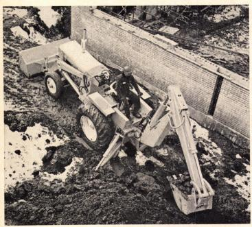
**Loader-tractor** has a lift capacity of 4,000 lbs, and a breakout of 6,500 lbs. Powered by gasoline or diesel, the unit has a working weight of 6,300 lbs. Five forward gears and one reverse are included. International Harvester, Chicago. Circle 229 on Reader Service card.
