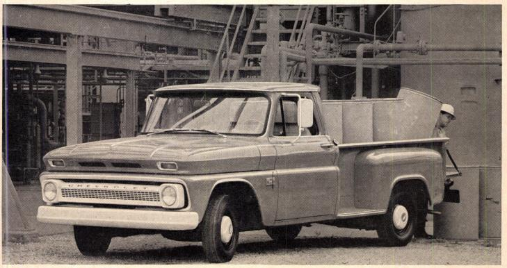
5 STEPSIDE MODELS—Available with 6½-, 8- or 9-ft. bodies. Feature flat interior body walls and handy side steps between cab and rear fenders. Same rugged planked floor construction with full-length steel skid strips as in Fleetside models. Maximum GVW ratings from 5,000 to 7,800 pounds.
