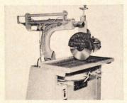
Radial saw has air hydraulic cross feed for automatic cutting. Uni-Point's blade always enters stock at the same point, thus eliminates need for blade adjustments. A blade cooling system is optional. Northfield Foundry, Northfield, Minn.
