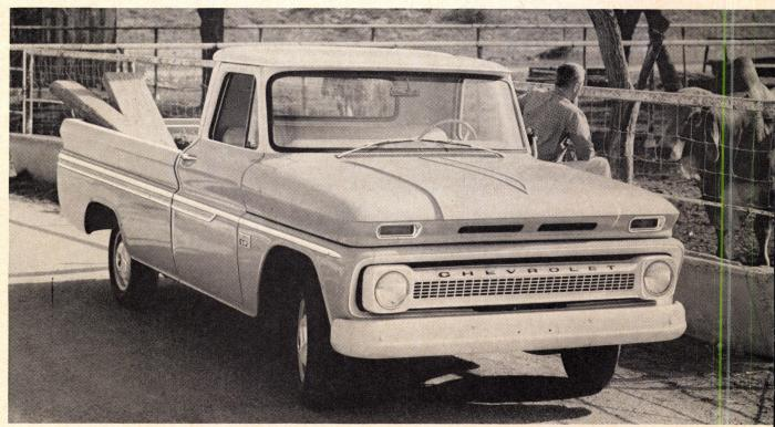
3 FLEETSIDE MODELS—Trim-lined Fleetside bodies are offered in 6½-ft. and 8-ft. lengths. Double-wall lower body side panels keep cargo dents from marring exterior appearance, and tough wood floor planking is joined by full-length steel skid strips. Maximum GVW ratings from 5,000 to 7,500 pounds.
