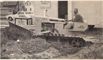
Crawler tractor has dozer attachment with hydraulic angle-tilt blade. Model 310 also has a loader attachment with a ¾-cu.-yd. bucket capacity and a 14′ backhoe with a 190° swing. Engine is gas or diesel fueled. Case, Racine, Wis. Circle 244 on Reader Service card.
