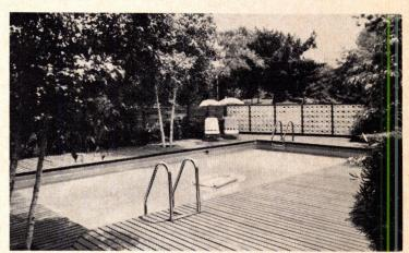
**Steel-walled pool** with vinyl liner slopes down from a wide shallow end to a narrow deep end. Seven sizes are offered from 16' x 32' (with depths of 3'4" to 5') to 20' x 40' (depths of 3'4" to 8'). Major Pool, South Kearny, N.J. Circle 155 on Reader Service card.
