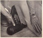
Finish nailer automatically nails and countersinks 1½", 1¾" and 2" nails. Machine is said to increase productivity 50% over conventional methods. Model FN-83 is portable and air driven. Duo-Fast Fastener, Franklin Park, Ill.
