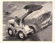
**Shovel loader** has a single-arm boom with a lift capacity of more than 3¾ tons. Four-wheel drive for power and traction and front-wheel steering for road-speed safety are included, says the manufacturer. Massey-Ferguson, Detroit.
