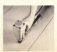
Lightweight stapler is designed for gypsum lath applications. Magazine carries over 140 16-gauge 7/16" crown staples in lengths up to 11/8". The 4-lb. Model C is said to be suited for overhead work. Spotnails, Rolling Meadows, Ill.
