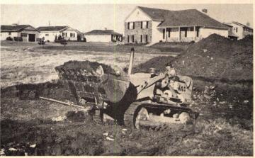
**Track-type loader** has pedal steering for increased operator efficiency, says the maker. Model 955 also includes planetary power shift transmission and automatic bucket controls. Nine bucket sizes with capacities to 23/8 cu. yds. are available. Caterpillar, Peoria, Ill.
