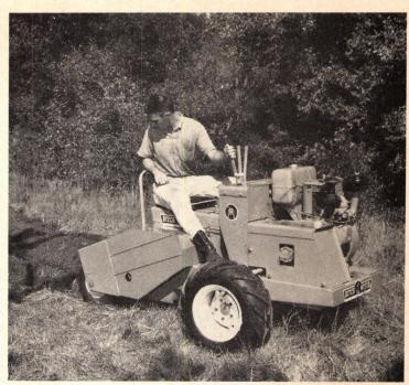
**Trencher,** called Model H12 Ditch Witch, has two-wheel drive that is easy to steer and operate, says the maker. The 12 h.p. model has a backfill blade designed for easy attachment. Charles Machine Works, Perry, Okla. Circle 241 on Reader Service card.
