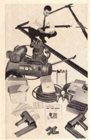
Truss system includes two pneumatic nailers, steel truss plates, truss nails, jig for truss part assembly, design manual, air compressor and accessories. According to the manufacturer, the system is low in cost. Bostitch, East Greenwich, R.I.
