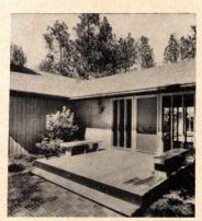
Rough sawn siding has a stain-type finish that combines preservatives, water repellents and pigment. Siding is durable and easy and inexpensive to apply, according to the manufacturer. Southern Pine Assn., New Orleans, La.
