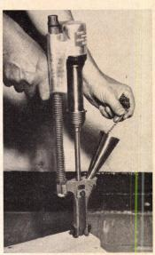
Nailer handles any bulk nail from 6d to 16d and drives as many as 50 nails per minute, according to the manufacturer. The unit weighs 7 lbs. Nails are dropped into the funnel and the trigger is pulled to operate. United Shoe Machinery, Boston. Circle 232 on Reader Service card
