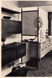
Room dividers have embossed translucent polystyrene insert panels framed in wood mouldings. Two designs are available—one with a circular and one with a diamond-shaped pattern. Both styles come in olive and amber. Panelboard Mfg., Newark.
