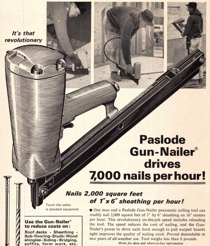
The Gun-Nailer drives regular 8d common or cooler and 6d common or cooler nails, with heads slightly modified to nest in clips. They are acceptable in FHA insured construction as equivalent to regular nails. They are *not* T-nails. It also drives galvanized nails 8d or 6d common; screw nails 2½" or 2" long; short (2½") 10d nails for diaphragm roof and shear wall construction.
